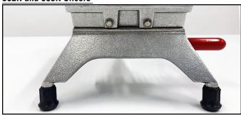
These slicers have two screws on each end that hold the blade assembly to the frame. To tension the blades, tighten the screws on the short leg end.
