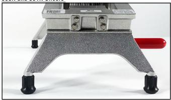
These slicers have four screws on each end that hold the blade assembly to the frame. To tension the blades, tighten the screws on the short leg end.
